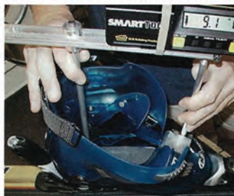
Below: ramp angle testing (left) and Campbell Balancer for binding position.
