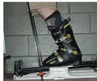
Below: ramp angle testing (left) and Campbell Balancer for binding position.
